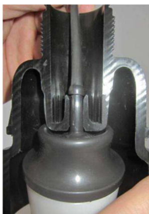
(Upper air valve part in cut sample view)
