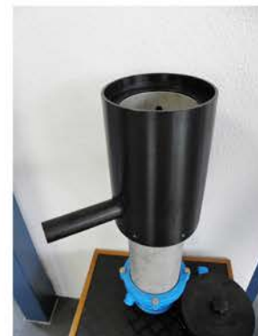
7. Adjust horizontal outlet into final position
