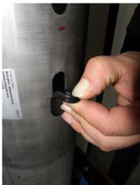
5. Remove sealing caps on both sides
