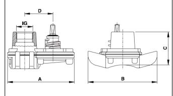
Material: Ductile Iron (GJS-400) with internal and external epoxy powder coating Medium: Potable Water
