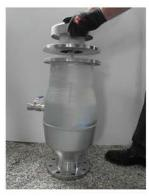
5.3 Lift complete function unit upward at the grip lugs. Place upright on the ground.
