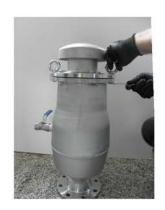
5.2 Lift flange with screen upward.
