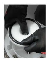
5.5 Clean and/or flush the slots of the air valve part.
