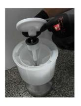
5.6 Remove diaphragm from the diaphragm bolt and check for debris and mechanical demages. Clean diaphragm from debris with water and towel. In case an exchange of the diaphragm is necessary remove the diaphragm from the diaphragm holder
