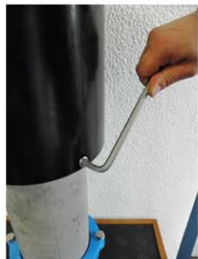
8. Screw down with an allen key to keep device in position
