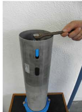
3. Loosen the screw
