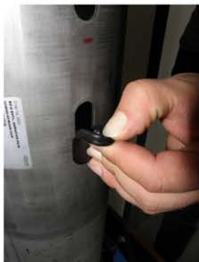
5. Remove sealing caps on both sides
